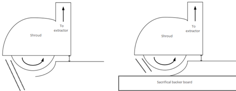
Figure 7: Use of sacrificial backer-board under material being cut to prevent dust release under material
